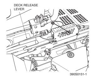
Figure 4-6. Deck Release Lever
